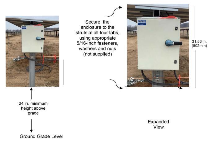
Fig. Power Assemblies PV Combiner Recommended Installation
