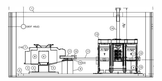
Fig. 4.1 PWA-COM-XXXX Major Component Identification and Location
